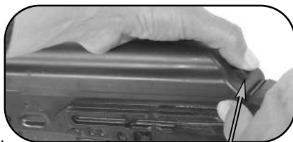
Spring loaded release button.
